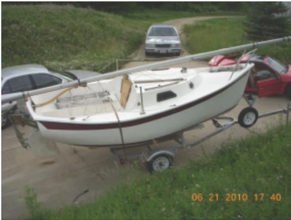
At left is skipper Jim Pardee's Seward Slipper 17. A very stable small boat that weighs in at 1,200 pounds including 400 pounds of ballast. Nearly 8 feet wide, it has a very roomy cockpit that easily accommodates the skipper and four passengers/crew.
